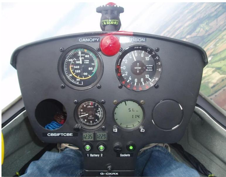
As you can see, a bank angle of 40 to 50 deg is not unusual. The panel may look sparse, but all the basic information is there; ASI and alti. to the left, here showing a typical circling speed of 50kt and approaching 3000ft. On the right are two variometers. They are showing a climb rate of 500fpm with an average climb rate in this thermal of 5.1kt so far...not bad for an unpowered aircraft!
